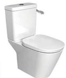
Tonic New Wave Close-Coupled Toilet (P-Trap) with disabled lever TF2102PD L690 x W400 x H810 mm
